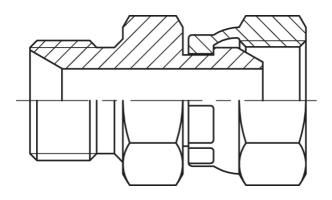
Product group Material Adjustable Bulkhead Shape Adapter type 780 Stainless Steel AISI 316 No Straight BSP
