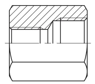
Product group Material Adjustable Bulkhead Adapter type Shape 780 Stainless Steel AISI 316 No BSP Straight
