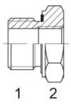
Product group Material Adjustable Bulkhead Adapter type Shape 780 Stainless Steel AISI 316 No BSP Straight
